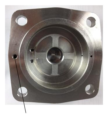
During re-assembling of the valve, make sure the large hole on the top half of the valve lines up with the hole on the bottom half of the valve
